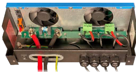
Inside the SmartSolar MPPT RS 450|100
